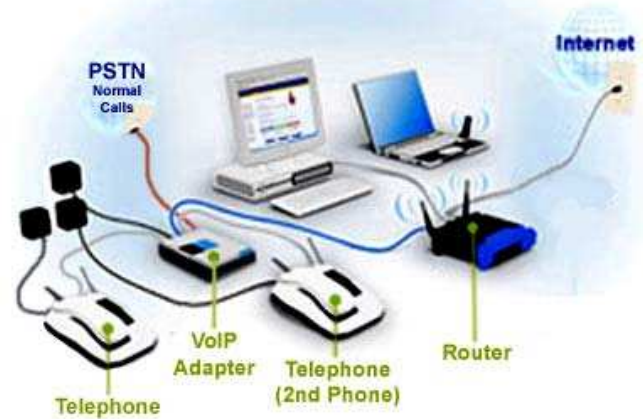
Figure 8. Displays an example of a VoIP setup utilizing an adaptor
