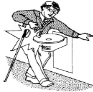
Figure 7 - Objects mounted above twenty-seven inches and that protrude more than four inches into the circulation path are hazards
