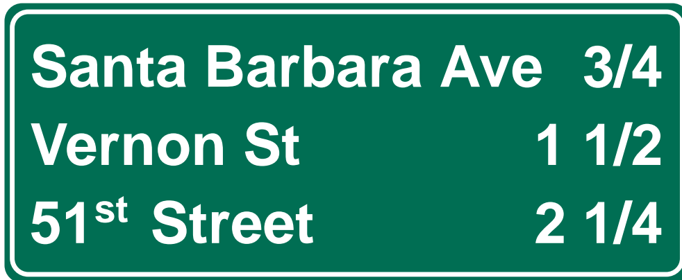
Figure 2E-22. Interchange Sequence Sign
